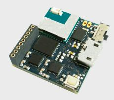
Presence of on-board floating point processing capability, along with four IMUs array, makes sensor fusion and motion processing possible within the module itself, which in turn results in very accurate motion sensing. It is also configurable as a wireless IMU, thanks to the onboard bluetooth module.
