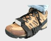
**Pedestrian Dead Reckoning (PDR)** is simplified with the footmounted MIMU22BLP/MIMU22BLPX. The device starts transmitting location data at every step, on receiving start command from the application platform. Based on this data, complete path is built in the application platform DaReX.
